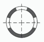
**Pipes slotted on two-thirds of their circumference (LP) –** pipes slotted along two-thirds of their circumference, installed on a sloped substrate. They are designed to absorb seepage water, groundwater, and surface runoff through the upper slots, while the closed lower part ensures efficient transport to the drainage system.
