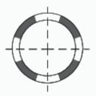
**Full-length slotted pipes (TP)** – – the most effective pipes for areas with permeable soil. Thanks to the slots distributed along the entire circumference of the pipe and the use of an appropriate filtration layer, they can absorb and transport not only seepage water and groundwater, but also water resulting from hydrostatic pressure from below.
