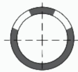
**Pipes slotted on one-third of their circumference (MP)** – pipes slotted along one-third of their circumference, intended for both partial soil drainage and collection. Their lower part remains closed, allowing for efficient water routing.
